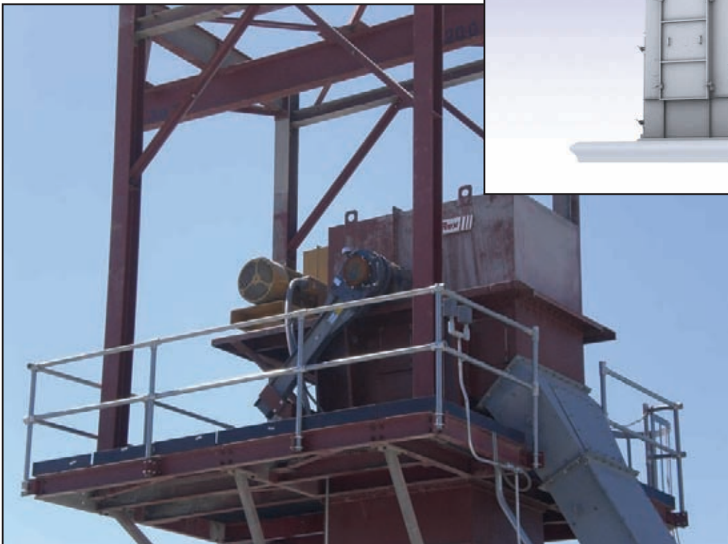
Rexnord Super Capacity elevators can be designed and built with large platforms and hoist frames that allow for easy maintenance access.
