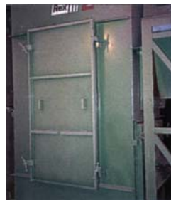
Large, easy opening access doors in the boot section are standard (and at other important locations as optional accessories) are for general maintenance and inspection.
