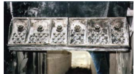
Rexnord patented belt splice has eliminated the problem of fastener fatigue breakage and related maintenance problems found in traditional clamping-type splices. Allows for easy and first re-splicing of belt using ordinary tools.
