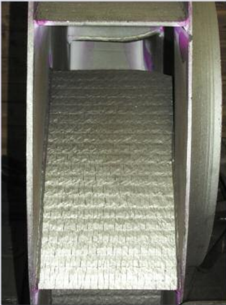
Hard surfacing of the blades...
