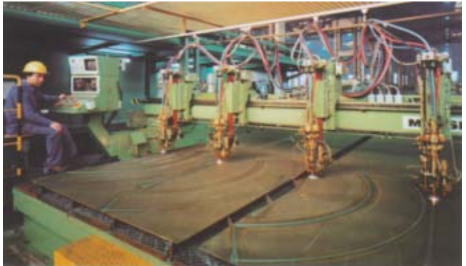
NC flame cutting machine, with punch tapes automatically produced via electronic data processor.
