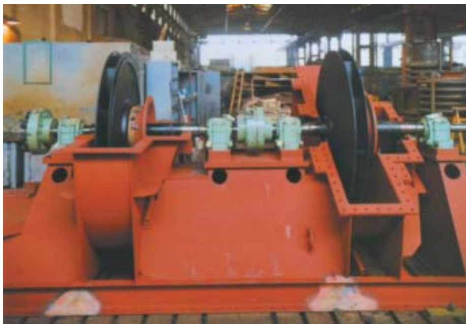
Two-stage F. D. fan for a waste gas combustor, the fan system consisting of two fans arranged in line with one common motor drive.
