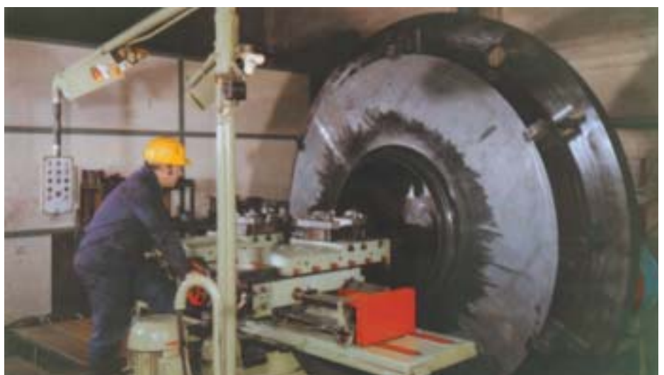
Metal spinning machine for radii of inlet nozzles, impeller side plates and spinning flanges.
