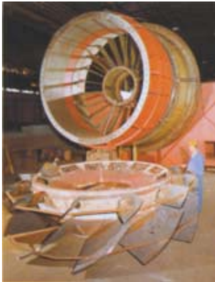
Axial flow impulse fan with slotted flap adjustment, shown during production.
