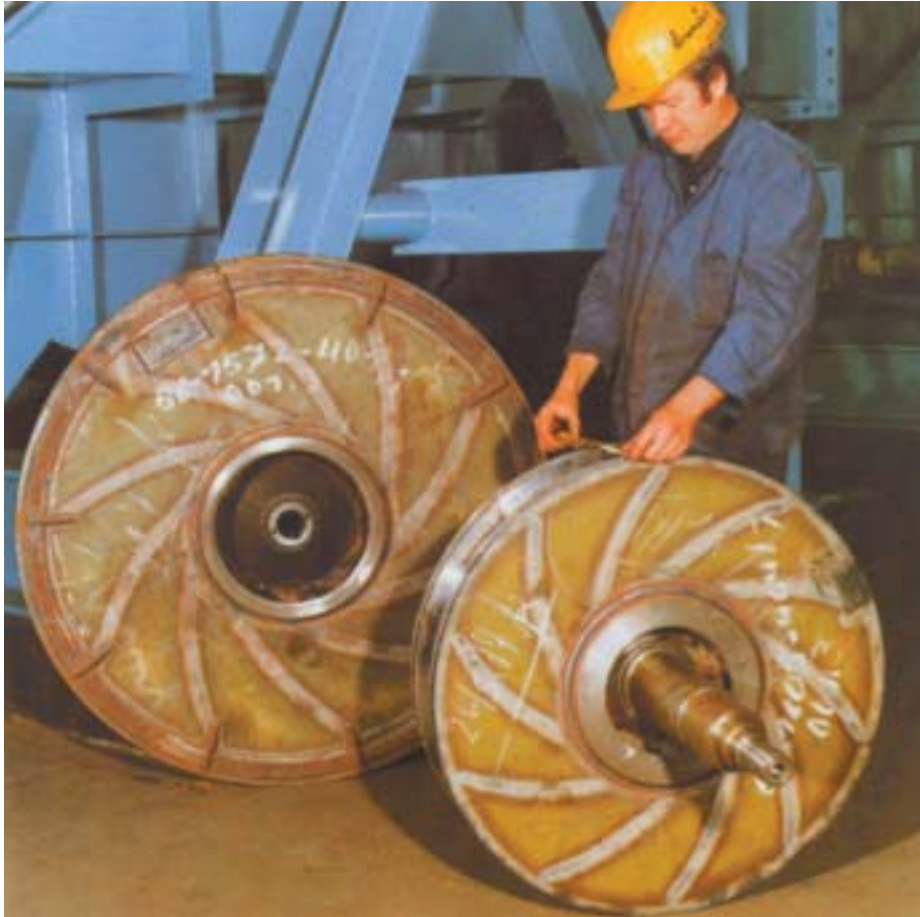
Left: Impeller for a single stage F.D. fan
