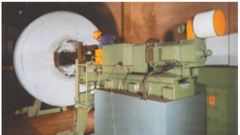
Balancing machine for fan rotors up to 30000 kg and 5000 mm Ø
