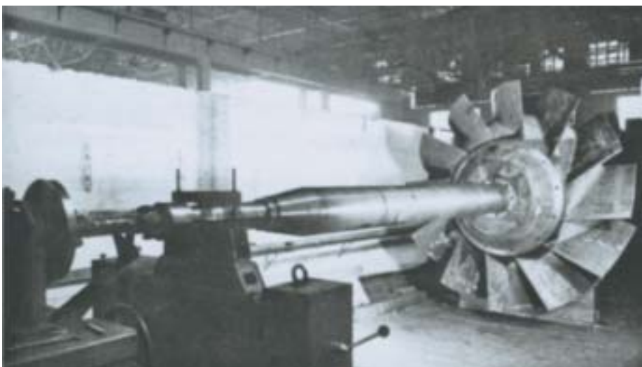
Impeller and shaft of an axial flow impulse fan during balancing operation.
